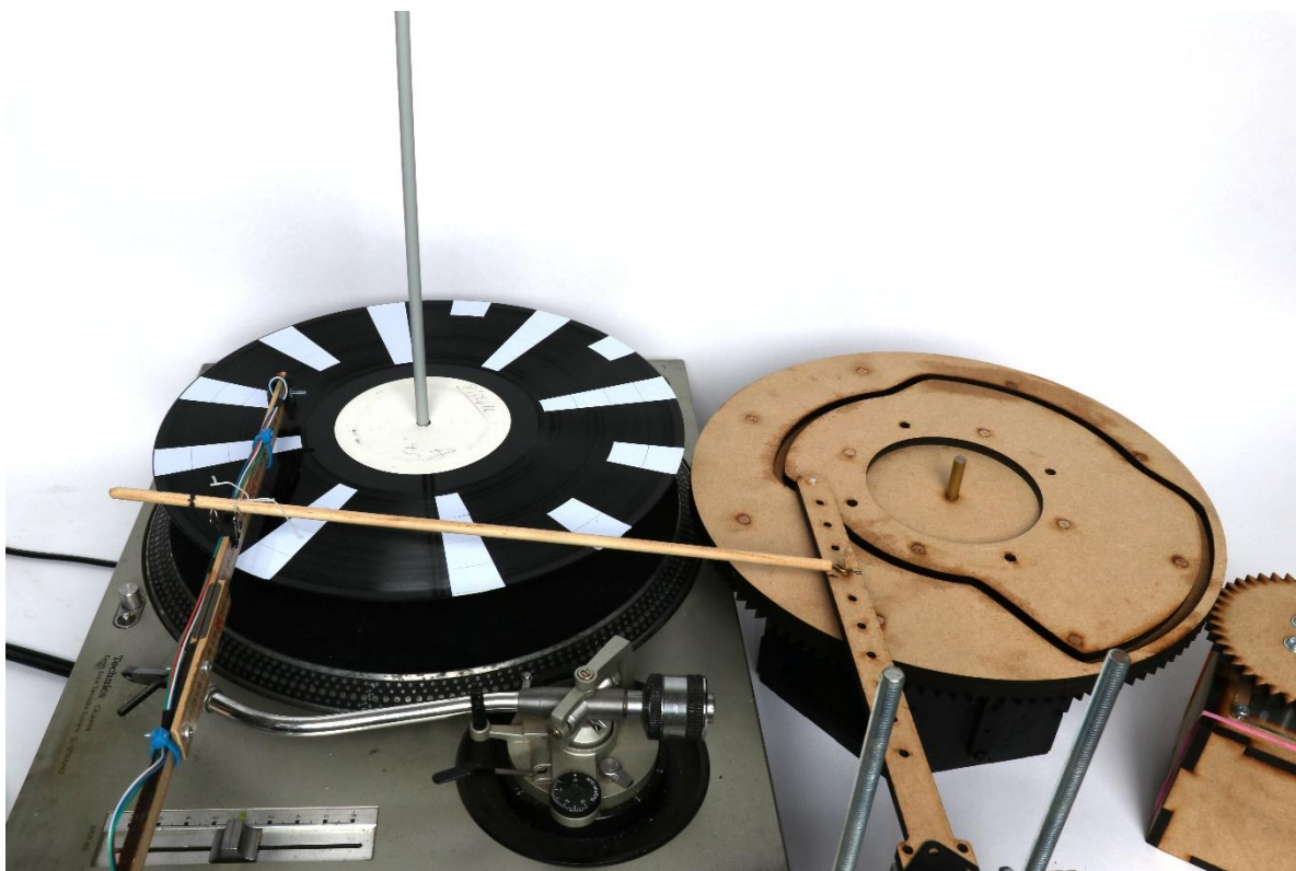
Image 6.12: Mechanical track changer.
