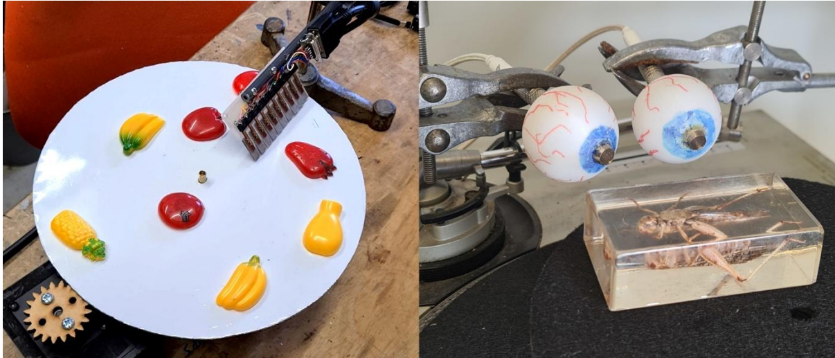
Image 6.7: Magnetic fruits and the MIDI Comb switch array. LDR sensors with an insect encased in resin.
