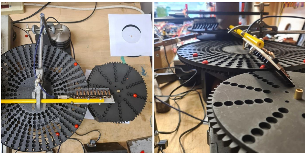
Image 5.6 cogs driven by the main turntable
