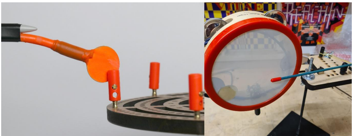
Image 6.9: Piezo trigger and drum with mechanical beater.
